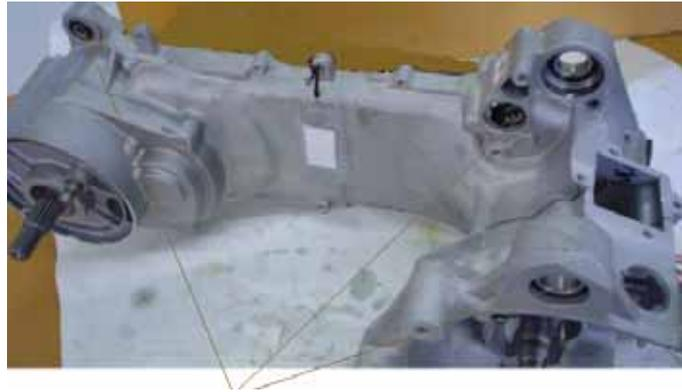
Install shock absorber bushing
