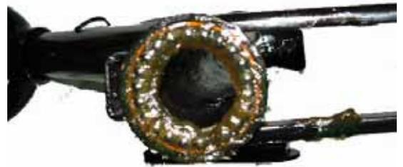
Tighten the steering outer race with special tool, then extrude it 1/8-1/4round.
