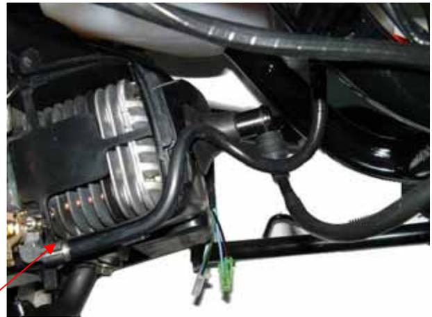
4. Remove rear brake cable adjusting nut ⑤
