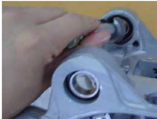
Install crankshaft (without bearings)
