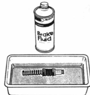
Reassemble and remount the master cylinder. When remounting the master cylinder on the handlebar, first tighten the clamp bolt for upside.
