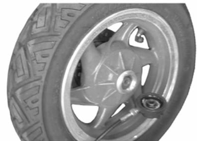
When installing this speedometer gear box, align the two driving pawls with the two recesses of the wheel hub. Tighten the nut with special tool.
