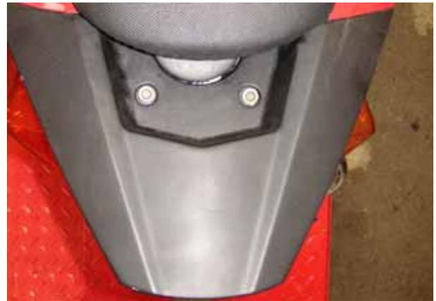
3. unlock oil pump cap and remove it, two tapping screw are exposed, remove them; remove tapping screw ⑨; then remove side cover ⑩
