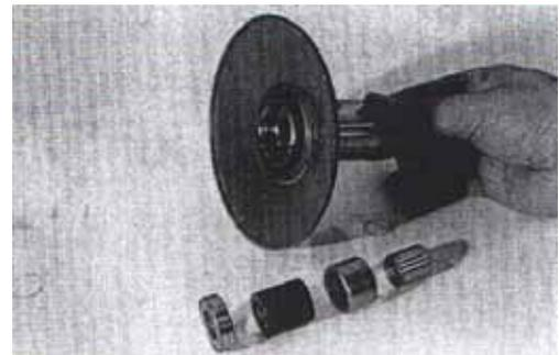
Remove the oil seal from the gearcase cover with the special tool.
